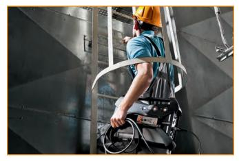
Combustion analyses in industrial processes vary widely.  $O_2$  and CO measurements are critical for proper combustion;  $NO_X$  or  $SO_2$  measurements are important for today's pollution control devices. Sometimes extreme concentrations are also encountered and unexpected. The testo 350's dilution system provides the protection and accuracy to continue working.
