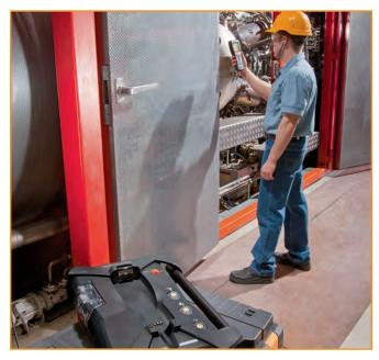
High output and low emissions are typical of turbines and as a result, you need an analyzer that is **especially equipped to handle low thresholds and still deliver the highest accuracy.** When you need to make critical control or warranty decisions, the 0.1 ppm resolution will provide the highest accuracy. The low  $\mathrm{NO}_{\mathrm{x}}$  and low CO sensors are ideal for the accuracy today's turbines demand.
