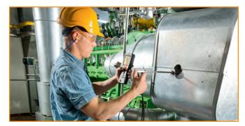
Rich-burn engine exhaust, when uncontrolled, can have wide concentration ranges and both CO and  $\mathrm{NO}_\chi$  can fluctuate significantly. The on-board CO dilution system will automatically set-up for optimum testing, perfect for a rich burn engine. Lean-burn engines have different exhaust characteristics, but  $\mathrm{NO}_2$  can make up a significant portion of the total  $\mathrm{NO}_\chi$  measurement. The 350 measures both NO and  $\mathrm{NO}_2$  for proper lean-burn engine set-up.
