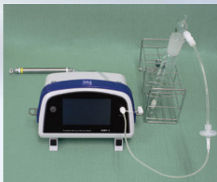
AQUA kit (option) For reducing vaporization mercury measurement
