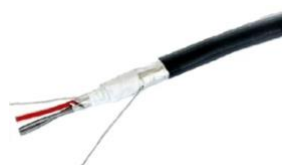
Integrated aluminium layer for reliable discharging of static chargings at the outer jacket
